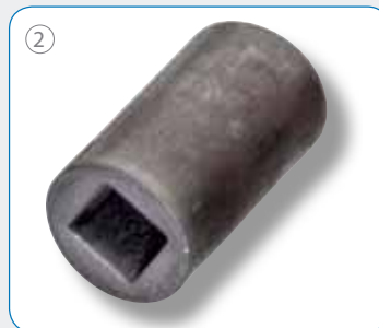
Hot forged in the forging press.
